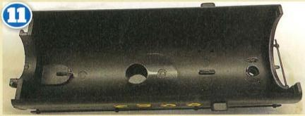
Clip out the plastic lugs from the inside of the saddle tank just to make it easier to reassemble later.
