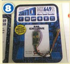
Turning our attention to the parts that are going to be fitted to the model we've opted for the wired MX649R version rather than the six pin MX649N. This decoder is pre-prepared with Digitrains 'J94' sound file, code ZS004A.
